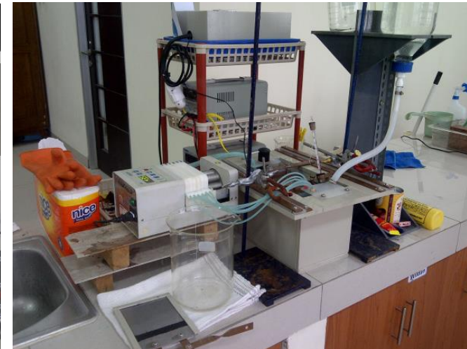
Metals electrorefining & electrowinning equipment
